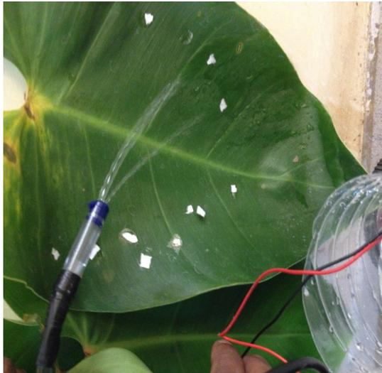
Fig. 9: Action of sprayer when pest is detected
