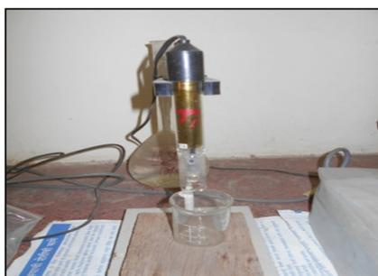
Fig. 3: Electric conductivity meter
