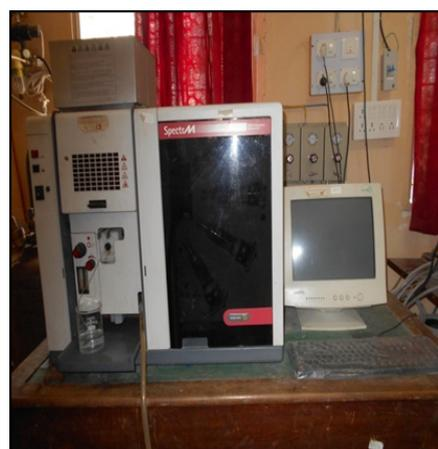
Fig. 1: Atomic Absorption Spectrophotometer
